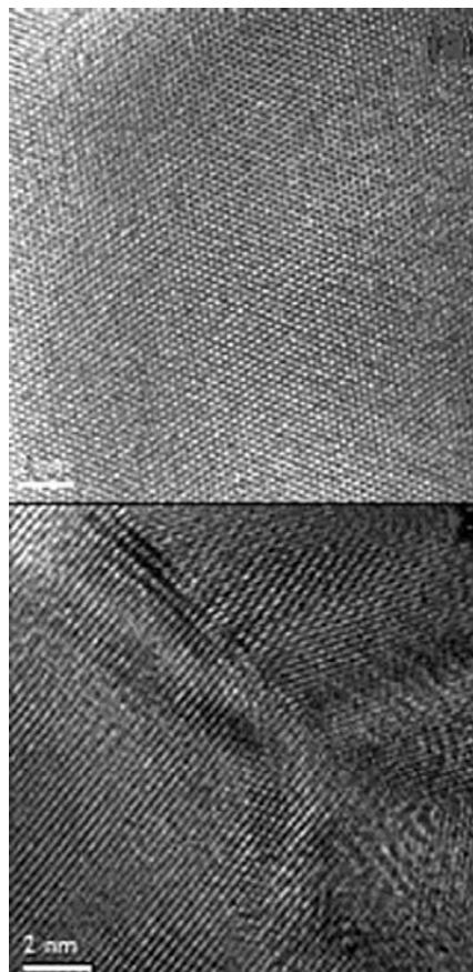
9 HRTEM images of ASAP plus 22 ppm silver phase, showing regions characterised by well crystallised single crystal (top) and distorted (bottom) lattices
